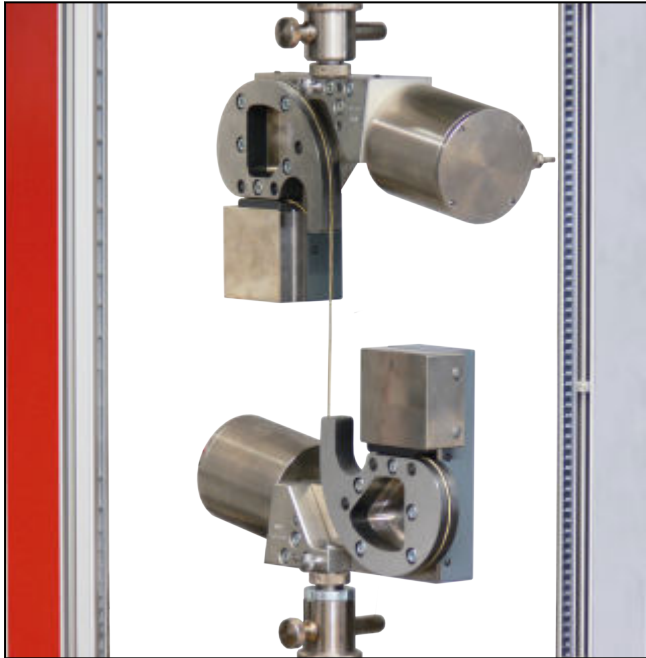
Capstan grips for steel tire cord to BISFA, type 8397, Fmax 10 kN
